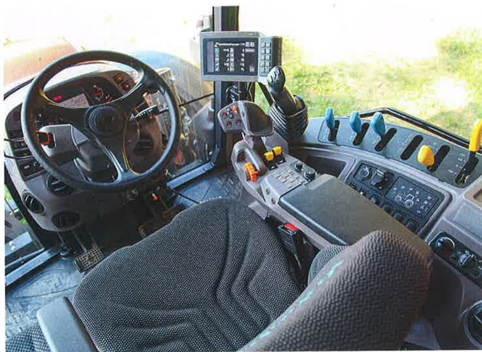
Armrest controls look after the gearbox and linkage. Mechanical spools and the front loader stick (this was not yet fully finished on our test machine) are located on the side console. Spool valve levers are not colour coded and, much like some other parts of the interior, feel a little cheap.
