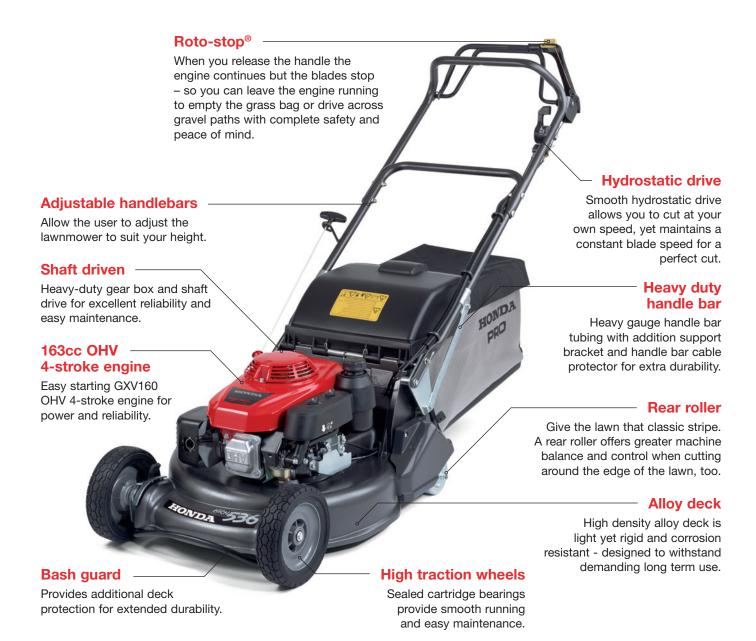
The HRH 536 QX is the tried and trusted professional's choice. Our HRH machines are engineered to meet the needs of the professional user, featuring a high density alloy deck, heavy-gauge handlebar tubing with additional support bracket and cable protection. The shaft drive and heavy-duty gear box makes maintenance both easier and less frequent. With the rear roller and a powerful and durable 163cc OHV engine, the mower drives along at a consistent speed for a perfect striped finish.
