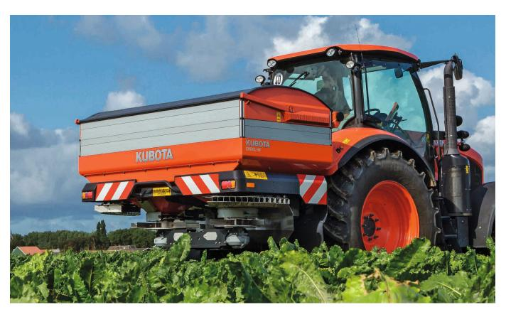
The DSM-W and DSX-W are weighing spreaders with the advantage of speed related spreading and high frequency automatic calibration. The DSM-W has hopper volumes from 1,100 - 2,000 ltires, can spread up to 28 metres and has one 10 tonne load cell. The larger DSX-W has more capacity with 1,500 - 2,800 litre hopper volumes, can spread up to 54 metres and it has four 5 tonne load cells positioned on both the front and the rear side of the spreader for the most accurate weighing.
