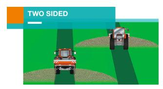
Border spreading plate Hydraulic operation of the border spreading plate from the tractor cab. The plate prevents fertiliser from reaching the field border by deflecting the fertiliser away from the border of the field.
