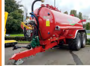
SlurryKat 14000 Tanker NEW, Rear Steer Axle, Sprung Drawbar Air & Hydraulic Brakes, Hydr Top Fill cap, Inspection hatch, 6" outlets
