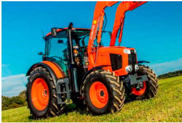
Kubota M115GX-III 24/24 Loader Tractor 123hp 40k, power shuttle, 540/1000 PTO, 6.1t lift, loader c/w bucket, 5 years Warranty available
