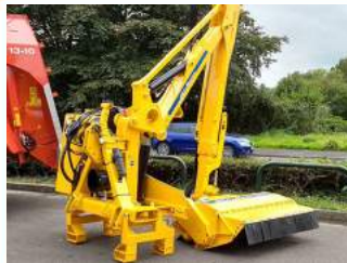
Shelbourne Reynolds HD760T Hedgetrimmer NEW, 6m LH Boom, Electrics, 3pt Linkage, Reversible head, Hydraulic Roller
