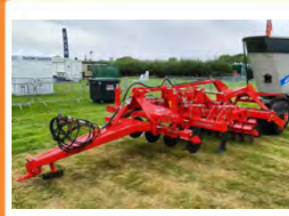
HE-VA Combi-Disc NEW, 3m working width, multi-purpose heavy duty cultivator, one pass subsoil, cultivate and consolidate. Finance Available
