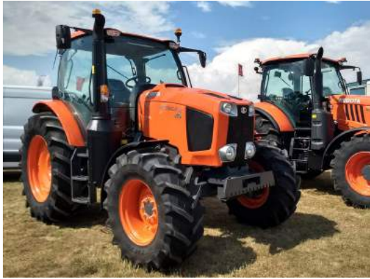
Kubota M135GX-III 24/24 40k Tractor NEW / Demo, 143hp, Power Shuttle, 540/1000 PTO, 6.1t lift, Front Axle Susp, 5 years Warranty available
