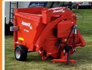
Jeantil PR4000 Straw Chopper NEW, semi-trailed round or square bales, Elec control box, hydr axle, 2.27m width
