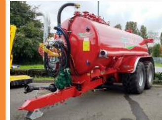
SlurryKat Tankers Options incl: Rear Steer Axle, 11000L pump, Sprung Drawbar, Air & Hydr Brakes, 8" Gate valve, 10 stud axles, Top Hatch
