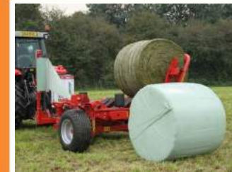
VICON BW2600J Trailed Wrapper NEW, DuoWrap twin film pre-stretcher, Joystick Controlled, Self Loading, Bales up to 1400kg, semi-automatic
