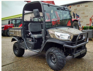
Kubota RTVx900 CAMO NEW, Road Legal, HST transmission, Roof, Glass Windscreen, Wiper Dual Seats, Nudge Bar, Hydraulic bed, Towbar (doors optional extra)
